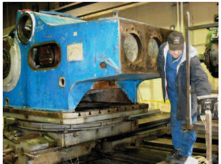
Collet Horizontal Boring Mill with Newall C80 3-Axes DRO. The Spherosyn scale is often exposed to dirt and oil because of the parts machined. Part Name: Mud Pump Housing. Machinist: Bobby Wright.
