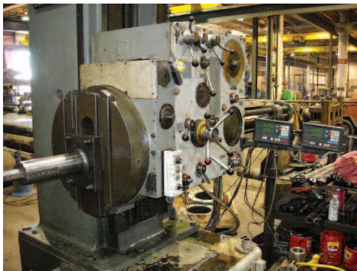
Droop & Rein Horizontal Boring Mill with twin Newall Topaz Mill 2-Axes DROs.
