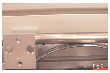
The scale will now be resting lower than the gauge position. Raise the support so that the scale touches the gauge. Refer to Fig.2.
